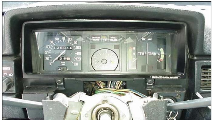
Now you can concentrate on the front of the dash. Start by removing the **two Phillip's screws** that hold the plastic cover on top of your steering column. Lift up and pull the cover toward you to remove. The photo shows the cover already removed.
