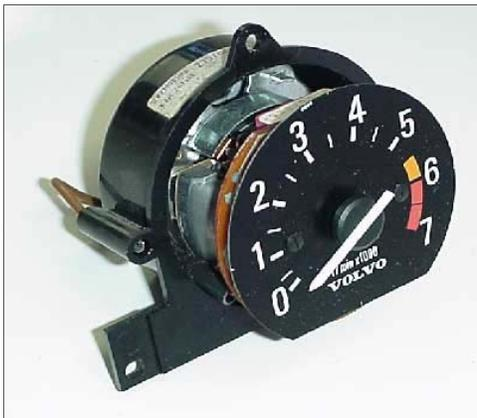
Gently grasp the needle with your fingers at the **center**. Twist the needle counter-clockwise. It will give a slight amount of resistance, so **don't put pressure on the needle pointer as it can break off**. While twisting the needle in a counter-clockwise direction, pull toward you. The needle will eventually pull off the small shaft. Re-installation is as simple as pushing the needle back on the shaft and pushing with your thumb.
