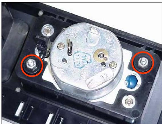
Looking at the rear of the clock/vent assembly, you will find two small nuts holding the clock in the plastic vent assembly. These nuts are **7 MM** on most clocks. Remove them.
