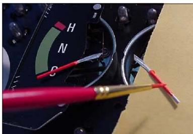
On the speedo and tach needles, use a bit a masking tape to keep from painting the black centers, or use a very gentle hand if you can.
