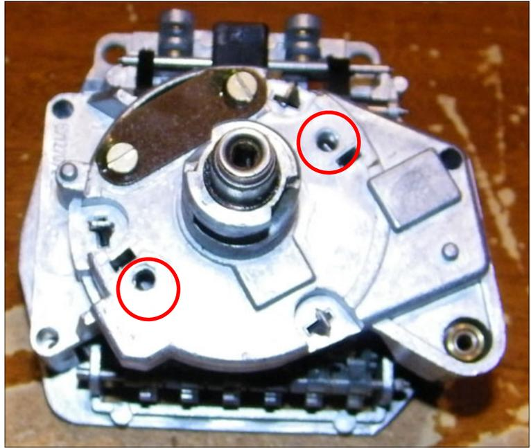
Now you should grasp the center round section of the needle. To remove the needle, you will turn it in a direction away from the stop pin at zero. Either direction is fine, just don't break the pointer arm on the pin. Some force will be necessary to release the grip on the shaft. Be very careful NOT to put pressure on the plastic needle pointer arm or it will break off.
