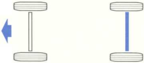
2. Axle-split system. This is a dual-circuit system which gives a little less than 50% efficiency should the circuit on the front wheels fail. The Ford Granada and Opel Commodore have this system.
