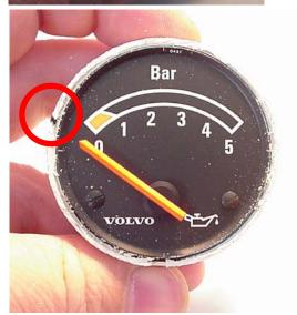
Notice that I placed a mark with a felt pen on the edge of the housing? This mark should be to record the position of the needle when at rest. It will be used later for lining up the needle when you reassemble. You should not skip this step.
