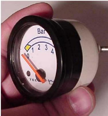
Now reassemble the gauge. If you used method #1, place the bezel ring back on and crimp the outside edge using a flat screwdriver.
