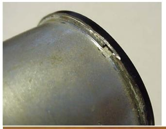
In the photo at left, you can see how a portion of the bezel ring has been trimmed away, exposing the lip on the gauge body.
