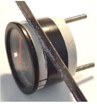
With a hack saw, slowly cut through the gauge housing, rotating the housing a little as you go. Be careful... don't allow the blade to go too deep; just allow it to break through the surface of the housing. Take your time.
