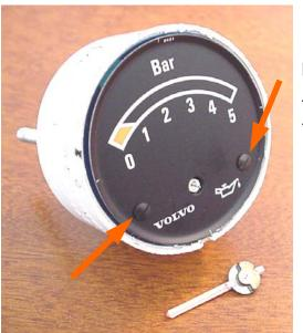
If your gauge face has these little screws (almost all do), use a proper fitting small screwdriver to remove them.
