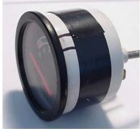
Measure about 1/4 inch away from the metal ring and place masking tape or electrical tape around the gauge for a cutting guide. A simple marker line works OK too.
