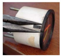
If your gauge has this plastic guide piece on the bottom, remove it. Simply pull it off with pliers.
