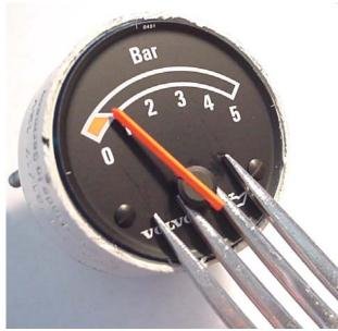
Now it's time to remove the needle. **Do not try to pull it off with your fingers or you will break it.** A simple kitchen fork does this job very well. **Be sure to pry straight up.**
