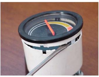
**NOTE:** If you are cutting an <u>OEM VOLVO 240</u> <u>Turbo Boost Gauge</u>, you will need to cut a little closer to the ring. Make your cut on this gauge about 3/16" from the ring.
