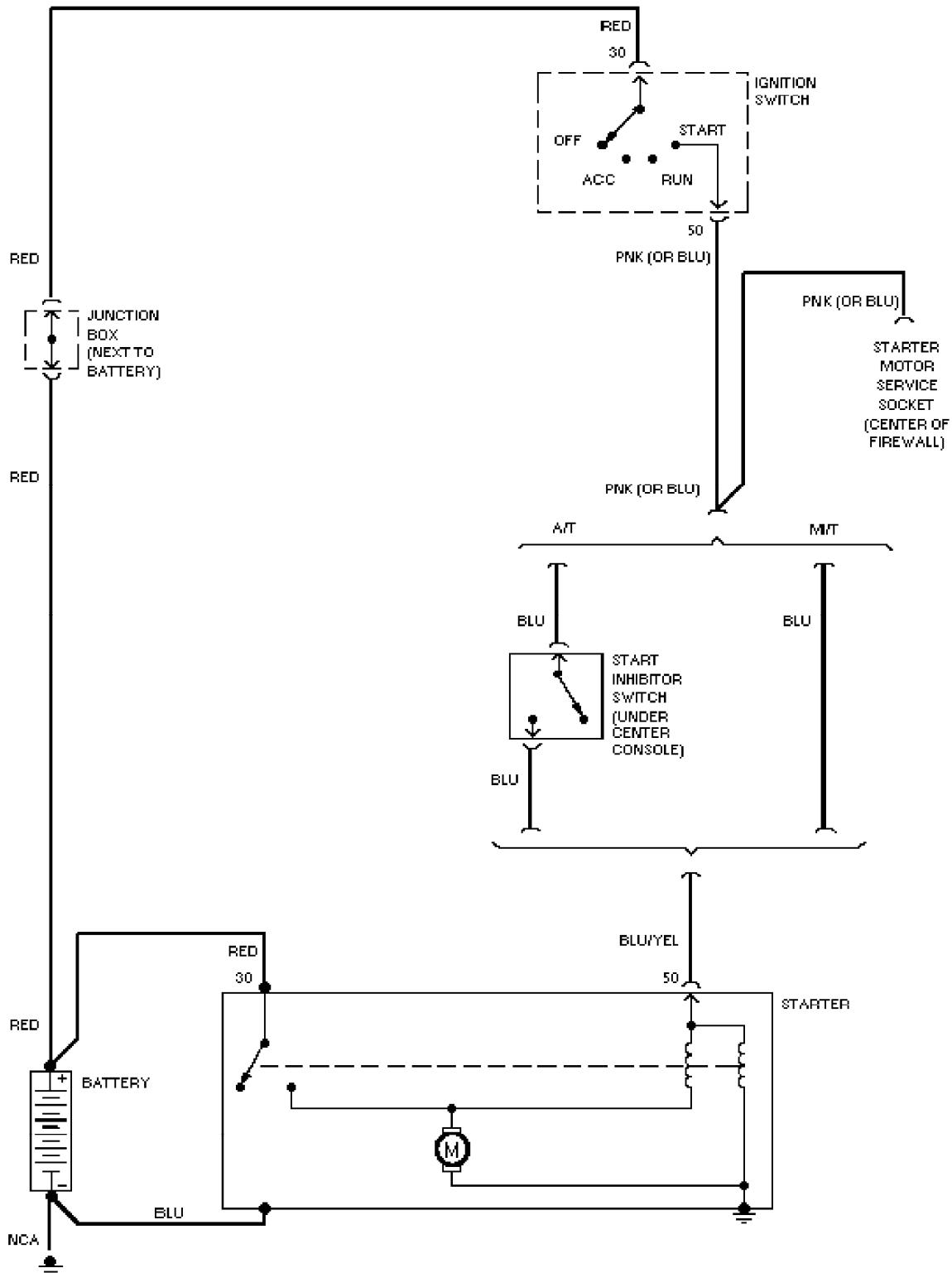
**SYSTEM WIRING DIAGRAMS**
