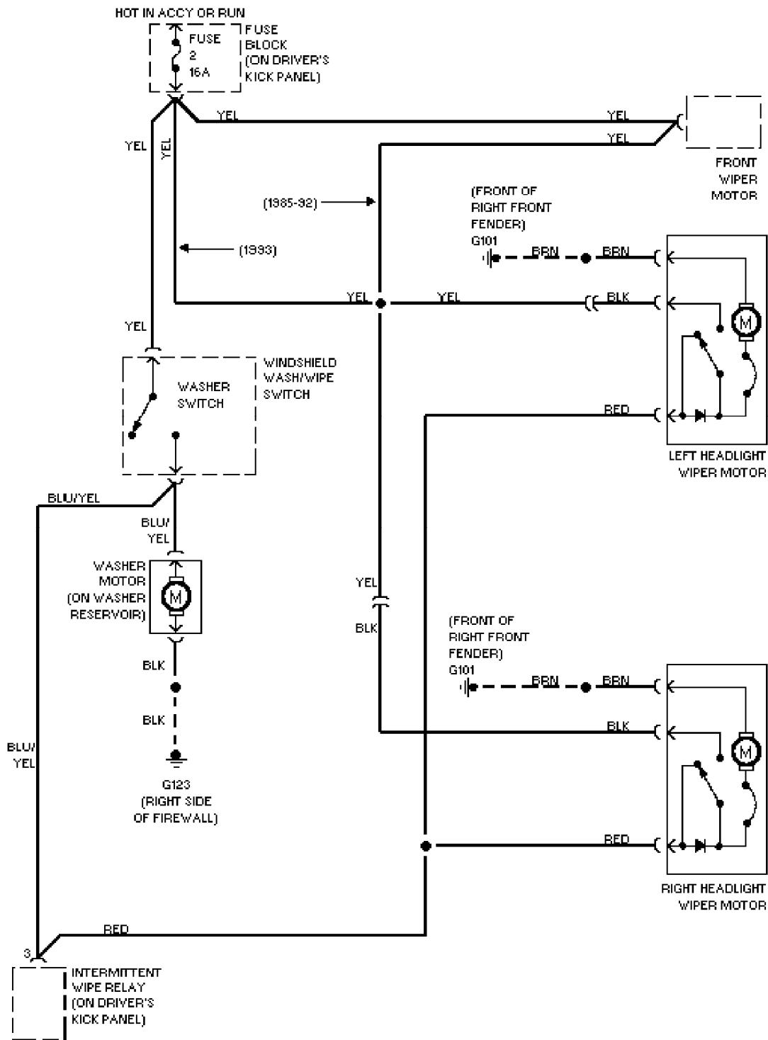
**SYSTEM WIRING DIAGRAMS**
