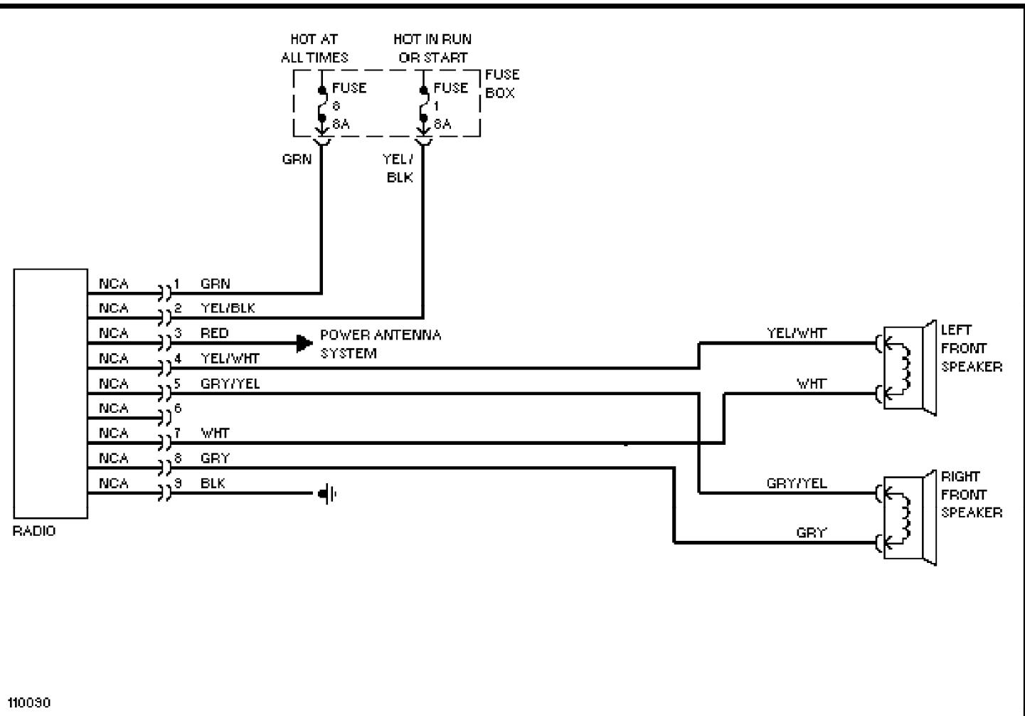
**SYSTEM WIRING DIAGRAMS**
