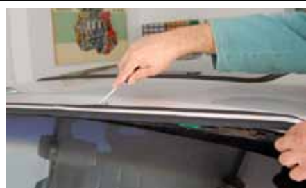
Disassemble the decorative frame of the windshield using a lever tool.
