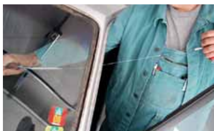
Lead the wire between the windshield and the body. Cut the window completely free.
