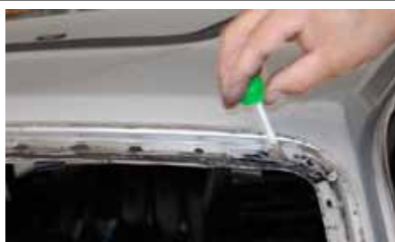
Apply the Butyl Primer to the bodywork.
