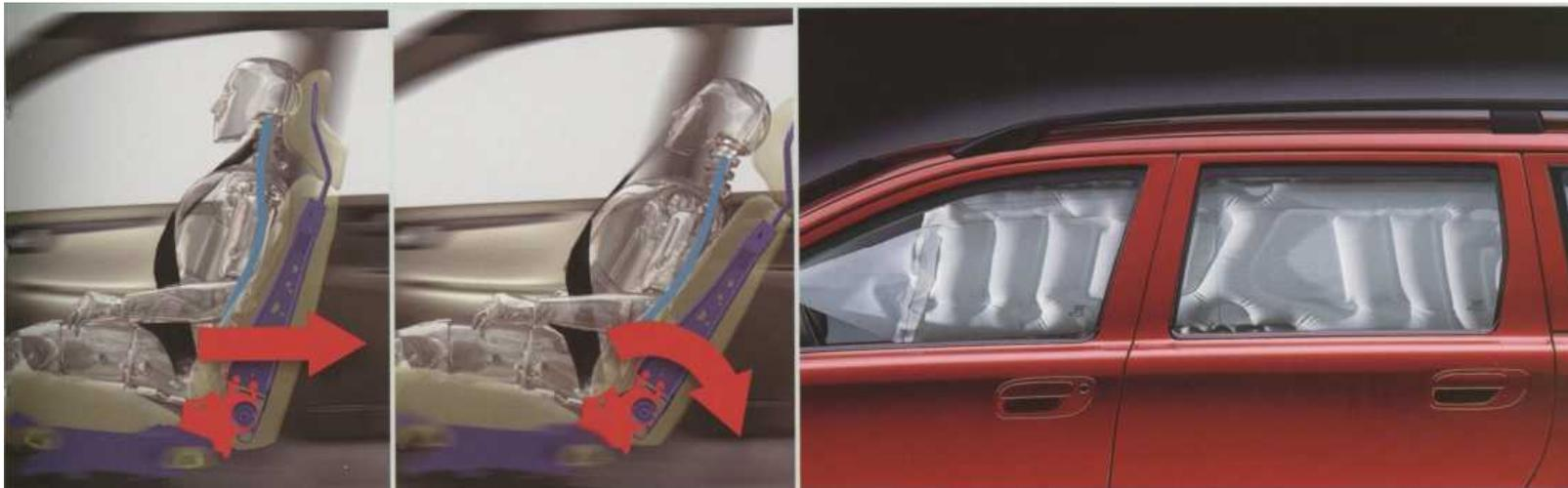
WHIPS (Whiplash Protection System) reduces the strain on the spine and neck in rear-end collisions. It is integrated in the front seats and is activated by a sufficiently severe rear impact.
