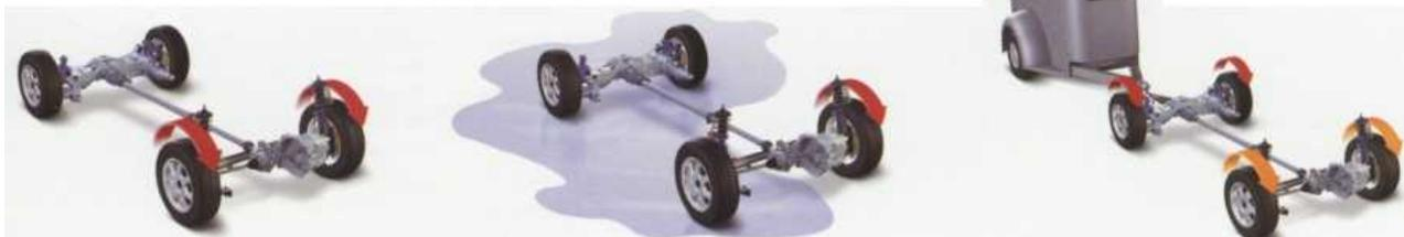
When braking, the car disengages drive to the rear wheels the moment you touch the brake pedal, preparing itself to maximise control and roadholding.
